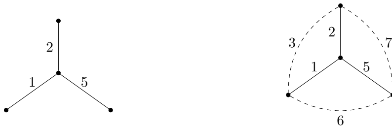
Figure 1: An example of the metric completion of a graph. The dashed edges are new edges added to make the graph complete.
