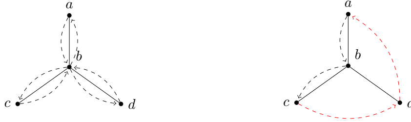
Figure 2: An example of shortcutting the in-order traversal of an MST starting from a . The red edges are the shortcut edges to avoid revisiting vertex b .
