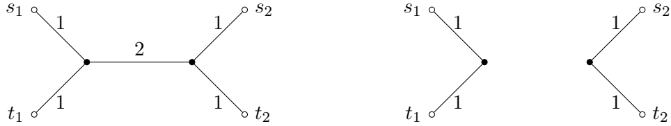
Figure 5: An example graph and its Steiner forest. The resulting subgraph need not be connected.
